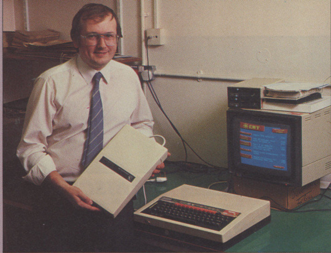
Jeremy Brayshaw, BBC Telesoftware Organiser with the BBC Micro system teletext adapter
